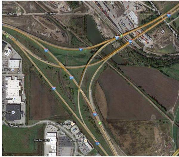
The project is replacing the westbound I-80 bridge over the RR yard with a wider, 3300' long bridge, a 1200' long ramp, and our portion...a 3675' x 32' flyover ramp bridge going from I-80 to southbound I-29.
